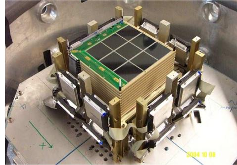
**Fig. 3** The MEGA prototype including Si strip detectors (D1) and CsI detectors (D2).
