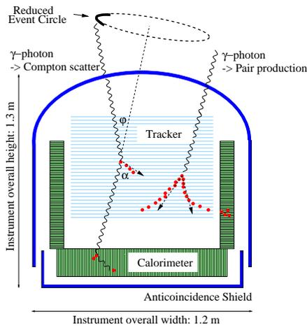
**Fig. 2** Schematic of the MEGA telescope showing the kinematics of gamma-ray interactions.
