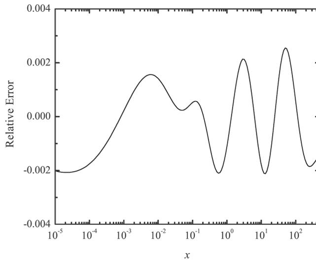
**Fig. 6** Relative error for the synchrotron function,  $F(x)$ , corresponding to the set of coefficients reported by Table 4.
