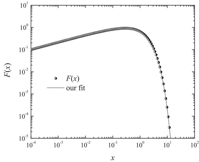
**Fig. 5** Synchrotron function,  $F(x)$ , together with its corresponding fit according to Eq. (6).
