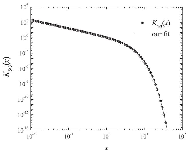
**Fig. 1** Modified Bessel function,  $K_{5/3}(x)$ , together with its corresponding fit according to Eq. (6).
