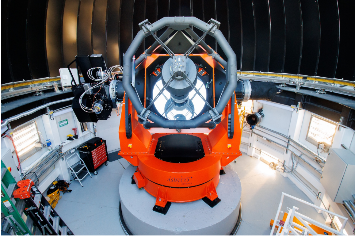
Figure 2. The COLIBRÍ telescope in its enclosure with the DDRAGO camera (left) and the OGSE test camera (right) mounted on its Nasmyth ports. DDRAGO is rotated to show the blue (upper) and red (lower) CCDs. The dummy derotator, used for balancing the instruments, is seen on the wall just to the right of the telescope.
