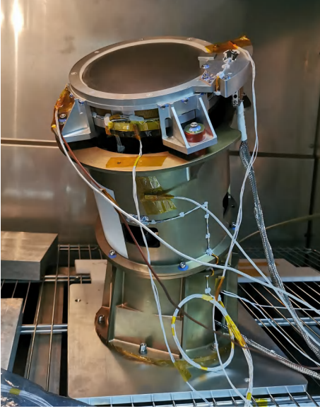
Figure 9. A GRD flight model unit undergoing thermal cycling testing. The unit is shown installed inside the thermal chamber, demonstrating the experimental setup used to verify the detector's performance under simulated space temperature environments ranging from +5°C to +35°C for 12.5 cycles, in accordance with the onboard product environmental testing requirements for the SVOM satellite.
