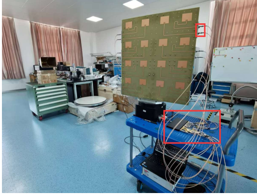
Figure 8. Analog beamforming network and pattern measurement platform.
