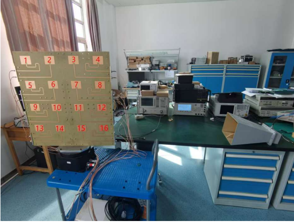
Figure 6. Experimental platform of beam calibration for PAF array.
