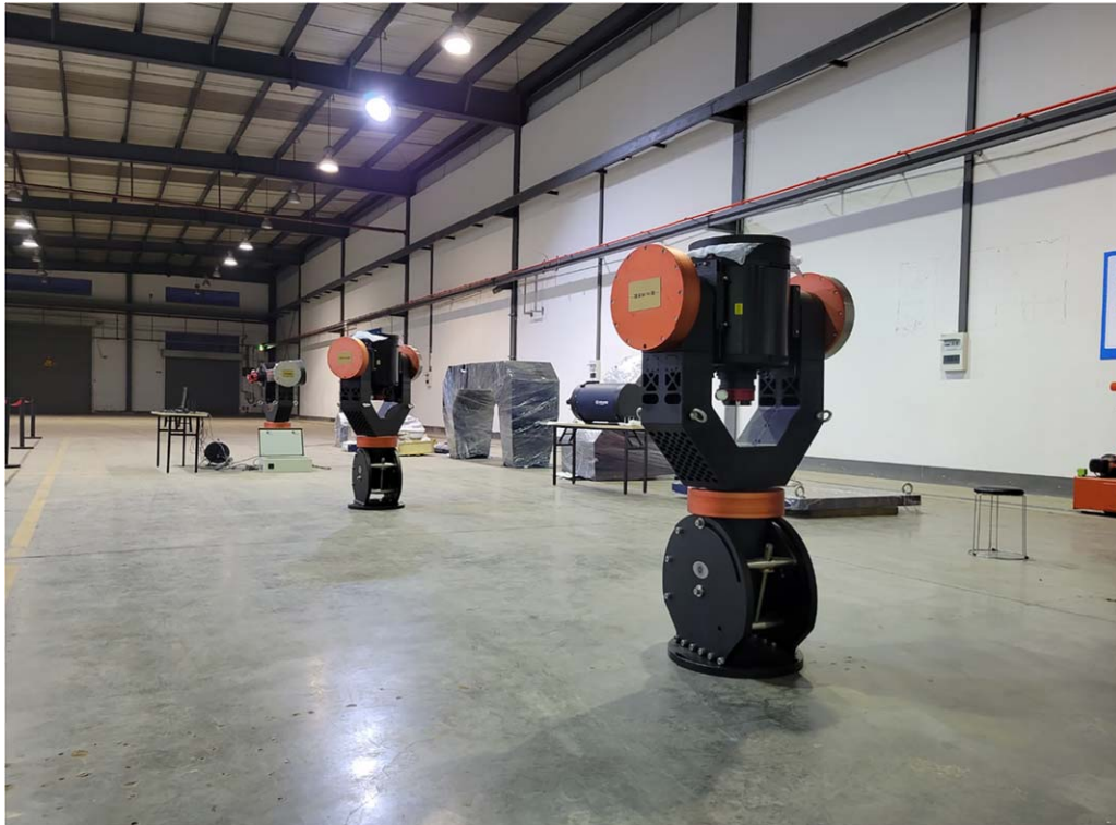
Figure 8. Equatorial mount of a Mini-SiTian Telescope Array in the factory.
