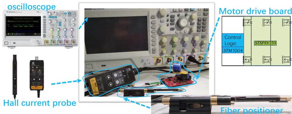
Figure 6. Experiment platform.
