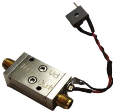
Figure 7. Photograph of CITLF3. The bias situation in this application are: 2 V of V_{ds} and 13.6 mA of I_{ds} .
