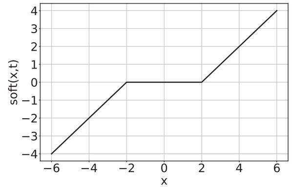
**Figure 6.** The soft thresholding function image, where the threshold value is 2.
