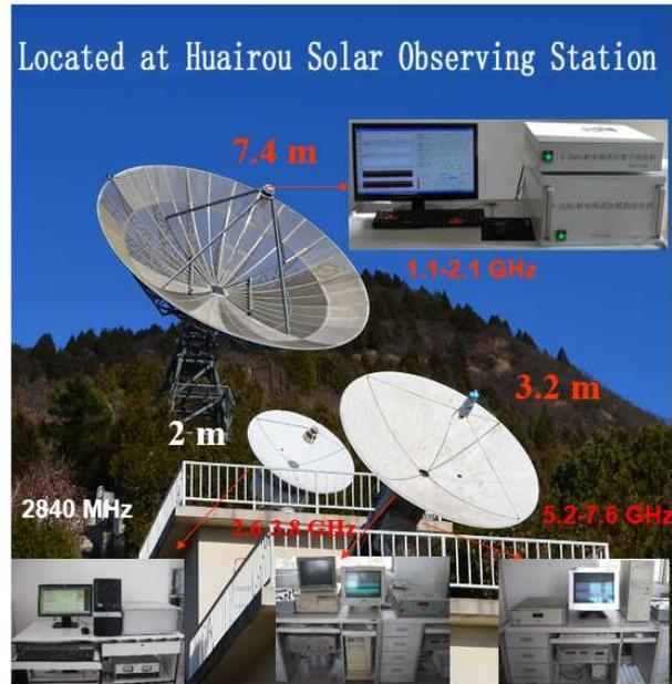
**Fig. 1** The Equipment of SBRS located at Huairou Solar Observing Station.
