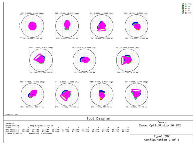
Fig. 6 The spot diagrams of optical system I at 40° zenith distance with the opposite direction FOV in Fig. 8. The circle diameters correspond to 232 μm (2 arcsecond).
