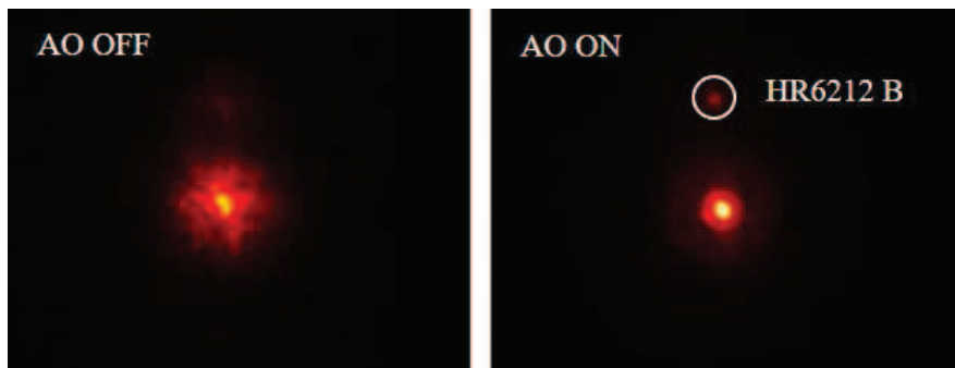
Fig. 8 HR 6212 A/B images before ( left ) and after ( right ) PAO correction at 3.5-meter ARC telescope.
