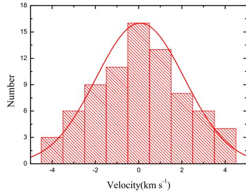
**Fig. 10** The statistic distribution of the radial velocity zero point for CES measured by radial velocity standard stars.
