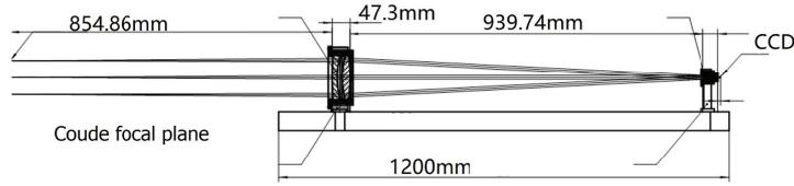
Fig. 1 The optical layout of the fine tracking feedback system for CES.
