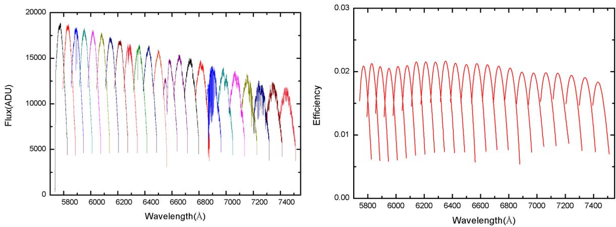
Fig. 8 The spectra of the standard star HD 23850 observed on 2016 January 18 and the derived total efficiency for CES based on the spectra at the spectral resolution of  $R = 32000$ .
