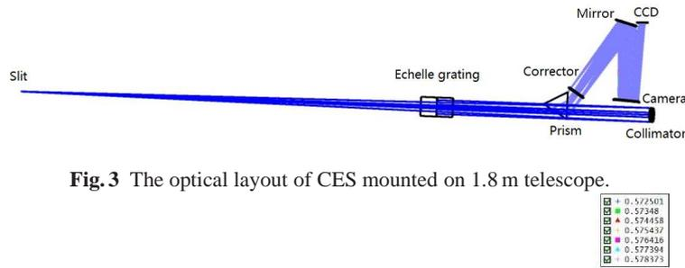
Fig. 3 The optical layout of CES mounted on 1.8 m telescope.
