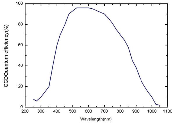
Fig. 7 The relation between the quantum efficiency of the PI CCD and the wavelength. In the wavelength coverage, the quantum efficiency begins to drop.
