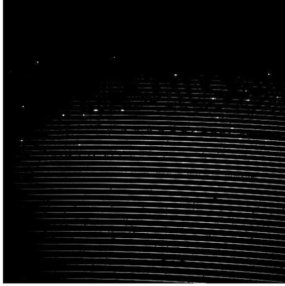
**Fig. 5** The measured spectral format on CCD of CES mounted on 1.8 m telescope. In the figure ThAr spectrum is superimposed on the stellar spectrum.
