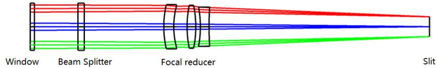
Fig. 2 The optical layout of the focal reducer designed for CES.
