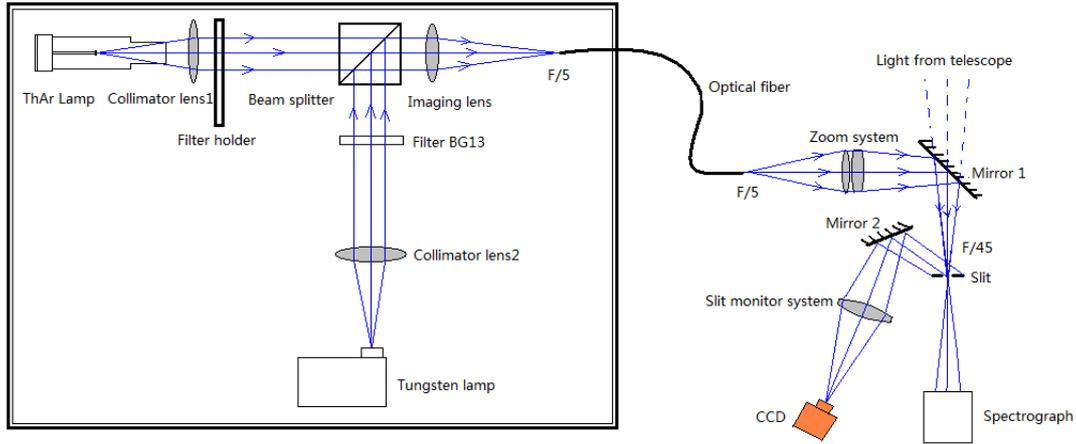
Fig. 6 The optical layout of the calibration and slit monitor system.
