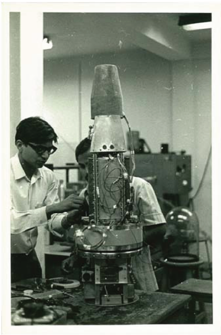
Fig. 1 The author ( on the extreme left ) engaged in testing the PCs for the rocket borne experiment at TERLS in early 1972 to measure X-ray spectra in 0.5–10 keV.
