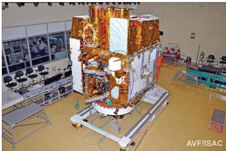
Fig. 10 Fully assembled ASTROSAT satellite ready for qualification tests in the Integration Laboratory of ISRO Satellite Centre, Bangalore in May 2015. The four science instruments can be seen on the top deck of the satellite with their view axes coaligned along the roll axis of the satellite.
