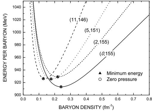
**Fig. 3** Density behavior of the energy per baryon with and without the inclusion of non-Newtonian gravity effects. Zero pressure (*open circles*) exactly corresponds to the minimum energy per baryon (the *triangles*).
