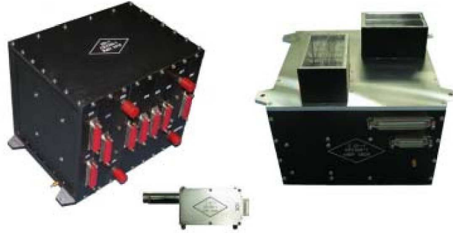
Fig. 1 The CE2XRS instruments, listed from left to right, are the electronic box, solar X-ray monitor and lunar X-ray detector. The photograph is from Peng et al. (2009).
