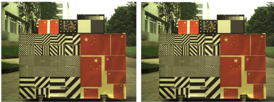
Fig. 8 Left: Before; right: After. Contrast between positive sample images before and after compression (MSE = 0.99, PSNR = 48.18).
