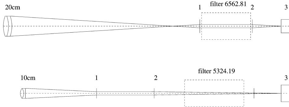
**Fig. 2** Optical scheme of full disk vector magnetograph (bottom) and full disk H $\alpha$  telescope (top), 1 – collimator lens, 2 – focus lens, and 3 – CCD camera.
