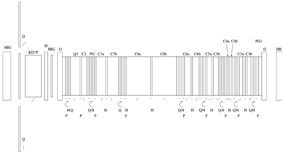
**Fig.3** Layout of birefringent filter at 5325.19 Å for the measurement of the magnetic field. ‘IF’ denotes interference filter, c1 – c7, calcite, Q1, quartz, G, glass, p, polarizers, PG, protecting glass, HIG, quarter-wave plate, H and Q, half and quarter-wave plates.
