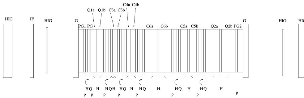
**Fig. 4** Layout of birefringent filter at 6562.81 Å for H $\alpha$  observations. The symbols are the same as in Fig. 3.
