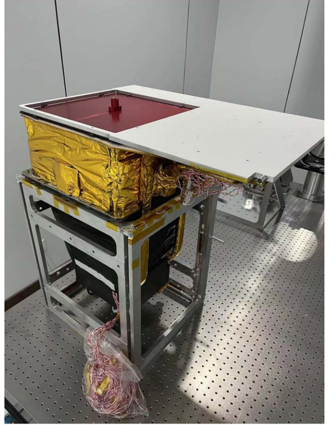
Figure 2. Picture of the LEIA instrument after engineering integration.
