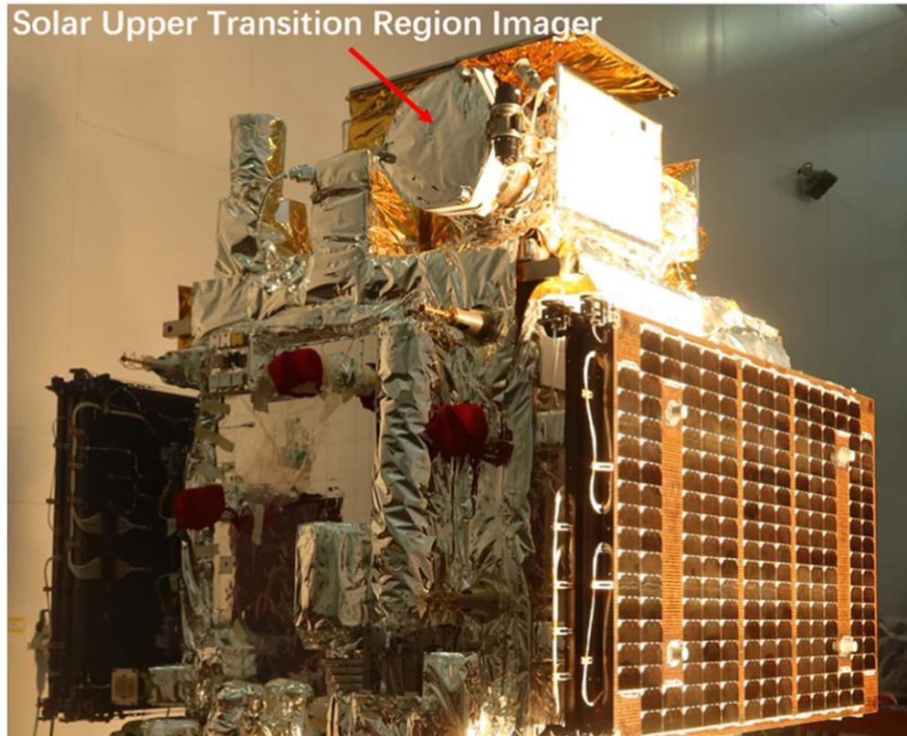
Figure 6. SUTRI installed on the SATech-01 Satellite.
