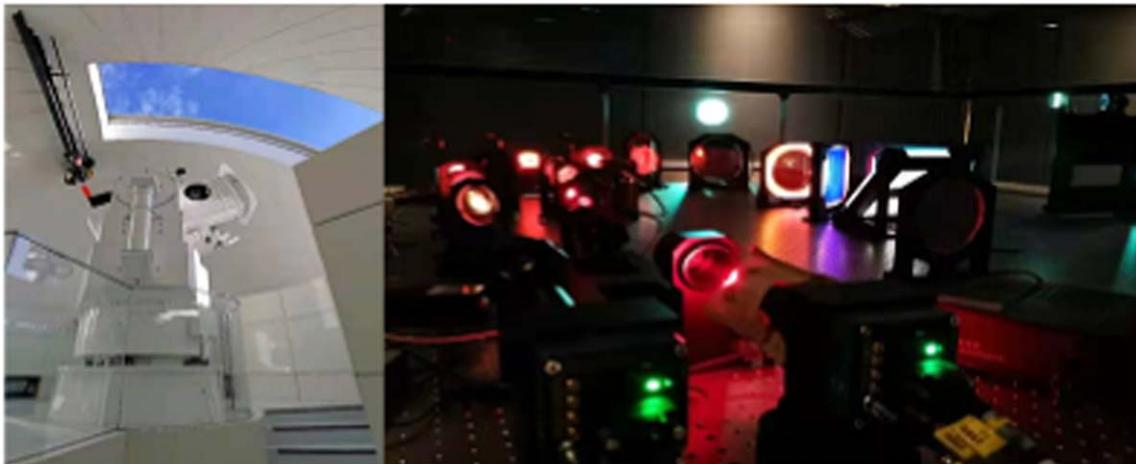
**Figure 1.** The 65 cm solar telescope and optical table with the adaptive optics system and two-channel high resolution imaging systems in the Coudé room.
