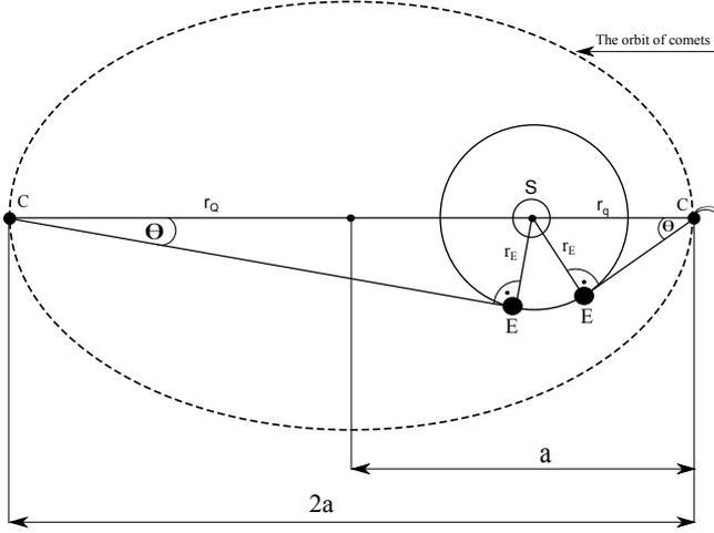
**Fig. 1** Graphical interpretation used to determine the phase angle. The individual symbols mean: S - Sun, E - Earth, C - comet,  $\theta$  - the phase angle,  $r_q$  - the distance of a comet being at the perihelion from the Sun,  $r_Q$  - the distance of a comet being at the aphelion from the Sun,  $r_E$  - distance of the Earth from the Sun ( $r_E = 1$  au),  $a$  - semi-major axis.
