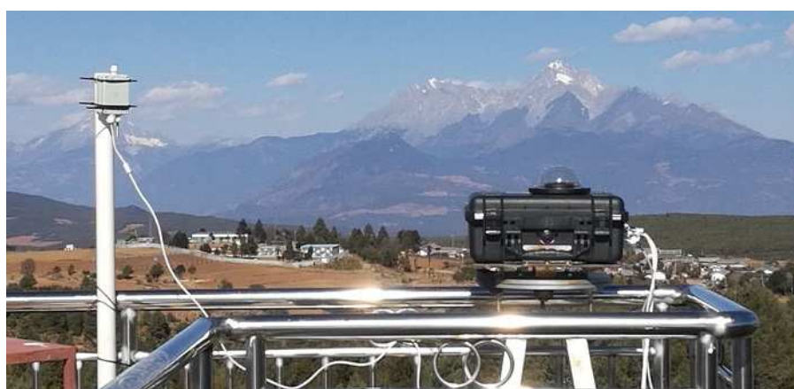
Fig. 5 All-sky Information Acquisition System on top of Water Tower ( Left : Cloud Sensor I; Right : All-sky Camera and SQM-LE inside the black box; Background: Haba Snow Mountain (left: 70 km far away, 5396 m high) and Jade Dragon Snow Mountain (right: 50 km far away, 5596 m high)).
