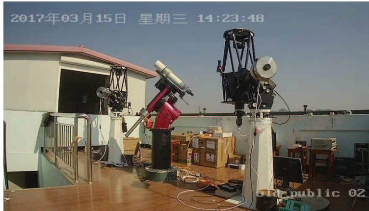
Fig. 10 Layout of two DIMMs.
