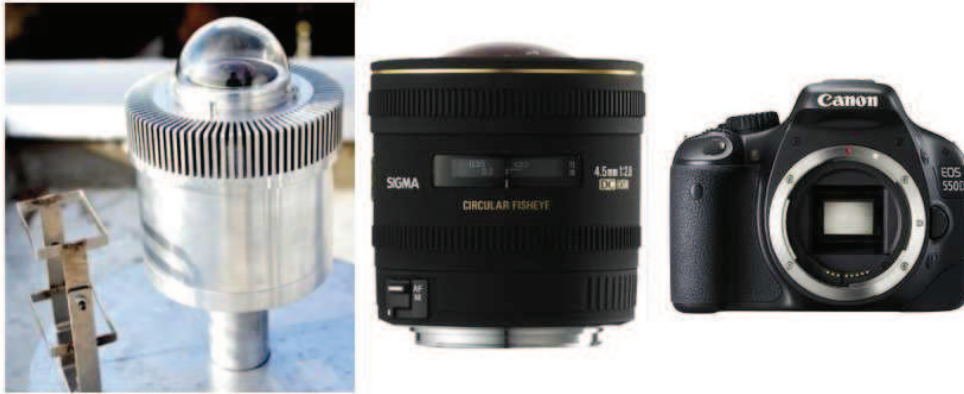
Fig. 1 Parts of the ASCA: sky quality ( left ), fish-eye camera ( middle ), and DSLR ( right ).
