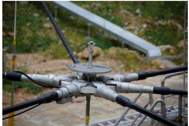
Fig. 2 2225 targets for laser measurement of the reflector system.
