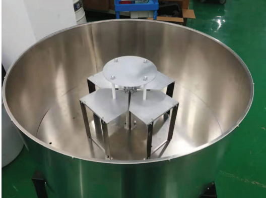
Fig. 6 The prototype of cross bow-tie dipole with back cavity.
