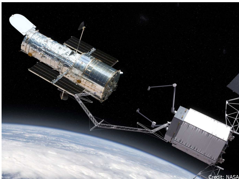
Fig. 3 HST has a coupling ring that will accept a robotic propulsion module that can de-orbit the telescope when it becomes non-operational.
