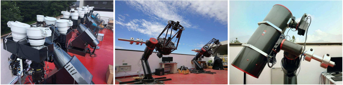
Fig. 9 ( Left ) The GWAC observation system mounted on its test bench at the Xinglong Observatory. O3 will be composed of four mounts. The total FoV of such a configuration is about 2000 sq.deg. The imaging time resolution is 15 sec for single frames. ( Center ) Two GWAC-F60 telescopes (60 cm) are employed to quickly confirm GWAC OTs and perform deeper follow-up observations if needed. ( Right ) A 30 cm telescope (GWAC-F30) will also be operated during the O3 campaign ( \text{FoV} = 1.8^\circ \times 1.8^\circ ).
