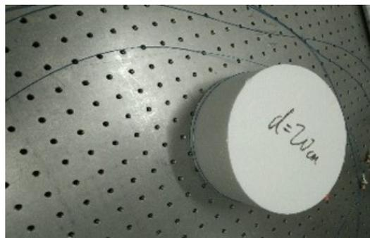
Fig. 13 The fiber bundle with a fixed bending radius at a distance of 1 m from the exit of the optical fiber bundle.
