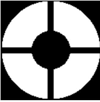
Fig. 4 The aperture geometry used in simulating the theoretical transfer functions and estimating the spectral ratio constants. The black regions indicate central obscuration and spiders holding the secondary. The white region signifies the useful aperture area.
