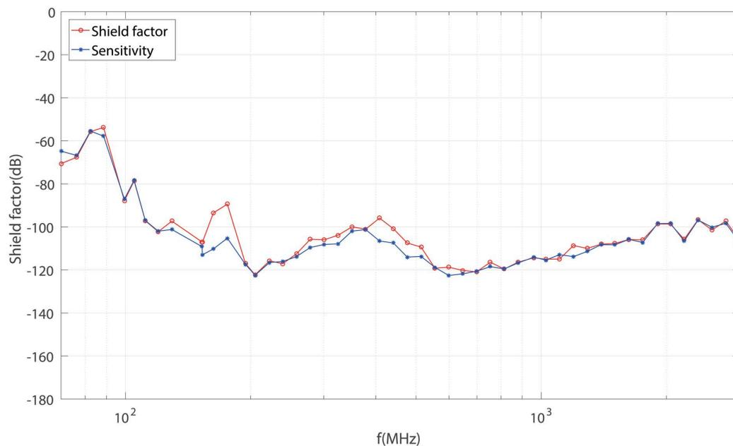
**Fig. 6** SE measurement result of one actuator based on the measurement method (Yue et al. 2015).
