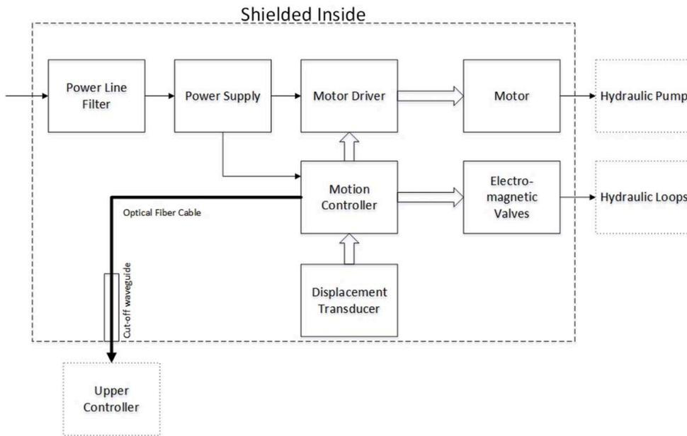
Fig. 4 A schematic diagram of the EMC design.
