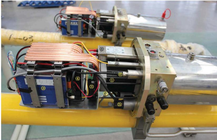
**Fig. 5** Electrical components inside the actuator. (1) Stepper motor; (2) Motor driver; (3) Actuator controller; (4) Power supply; (5) Electromagnetic valve; (6) Pressure-temperature sensor; (7) Wire for the displacement sensor; (8) Power line filter; (9) Cut-off waveguide.
