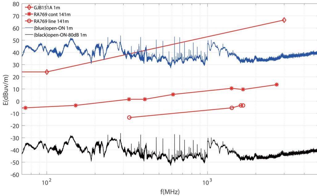
Fig. 3 Typical EMI from an actuator with an open enclosure measured in the anechoic chamber based on GJB151A RE102 with 80 dB reduction.
