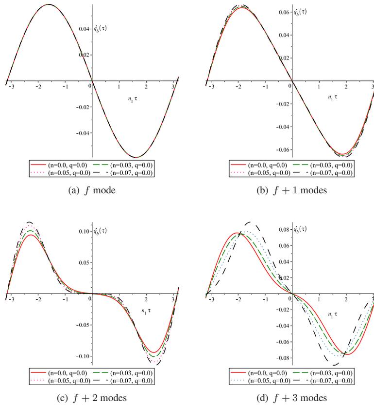
Fig. 10 Radial velocity curves of the rotationally distorted polytropic models with  $N = 3.0$  ( $n$  varies and  $q = 0$ ).
