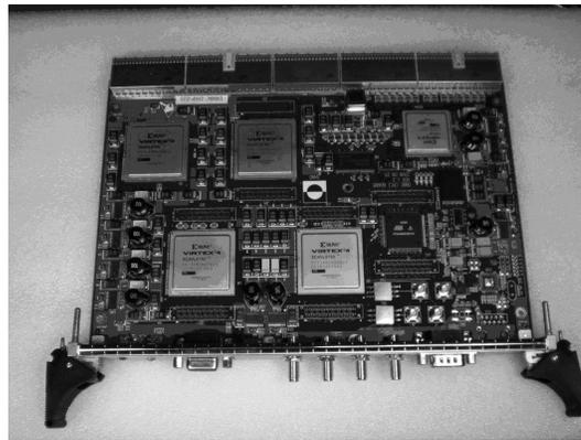
**Fig. 2** The digital signal processing board.
