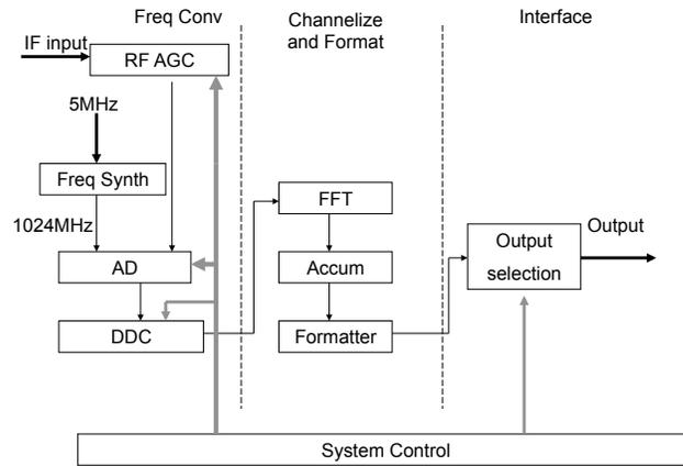
**Fig. 1** Schematic diagram of the digital pulsar backend.
