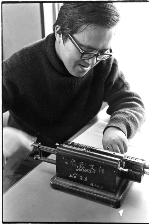
Fig. 1 The author demonstrates how to use a hand computer (Tiger calculator). The Japanese characters at the back of the computer say that this is property of Tokyo Astronomical Observatory. The photo was taken in around 1955.
