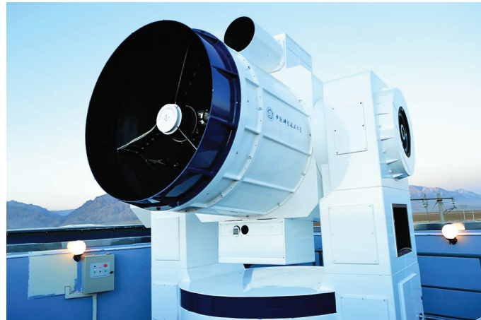
Fig. 5 The 1.2 m telescope system used for quantum communication and astronomical observation.
