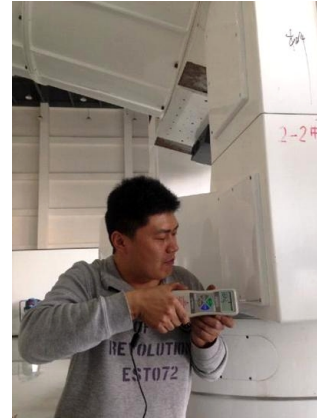
Fig. 9 Imposing some periodic disturbance torques via a dynamometer.
