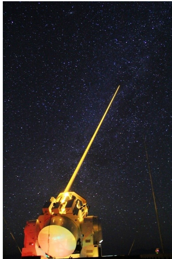
Fig. 2 A photo showing the sodium laser being launched into the sky.
