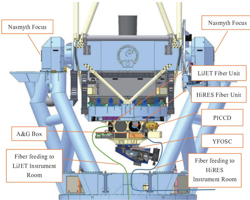
**Fig. 5** The instruments mounted on the Cassegrain A&G box. YFOSC is mounted on the straight-through focal plane. The PICCD, and fiber coupling units of LiJET and HiRES are mounted on the side ports.
