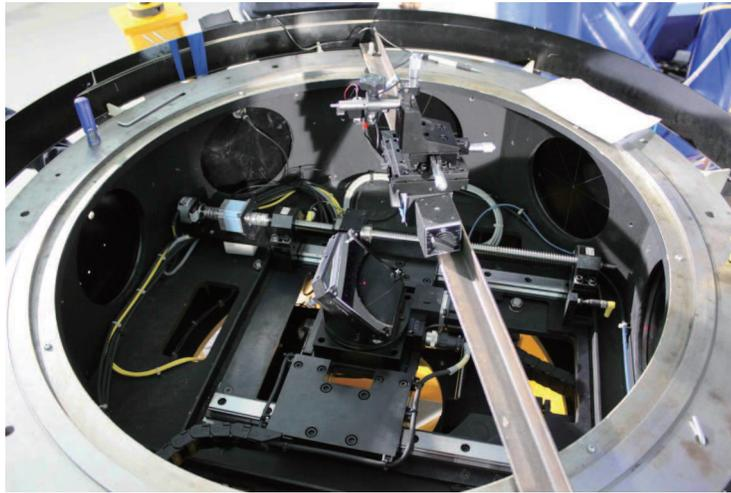
**Fig. 4** The folding mirror installed inside the A&G unit. To center and align the mirror, a reference laser beam was pointed along the optical axis of the telescope.
