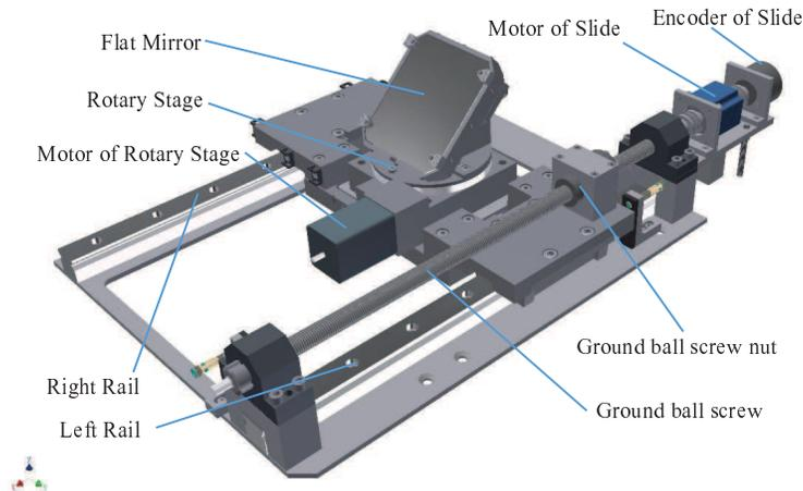
**Fig. 2** The mechanics of the tertiary mirror rotating and retracting.
