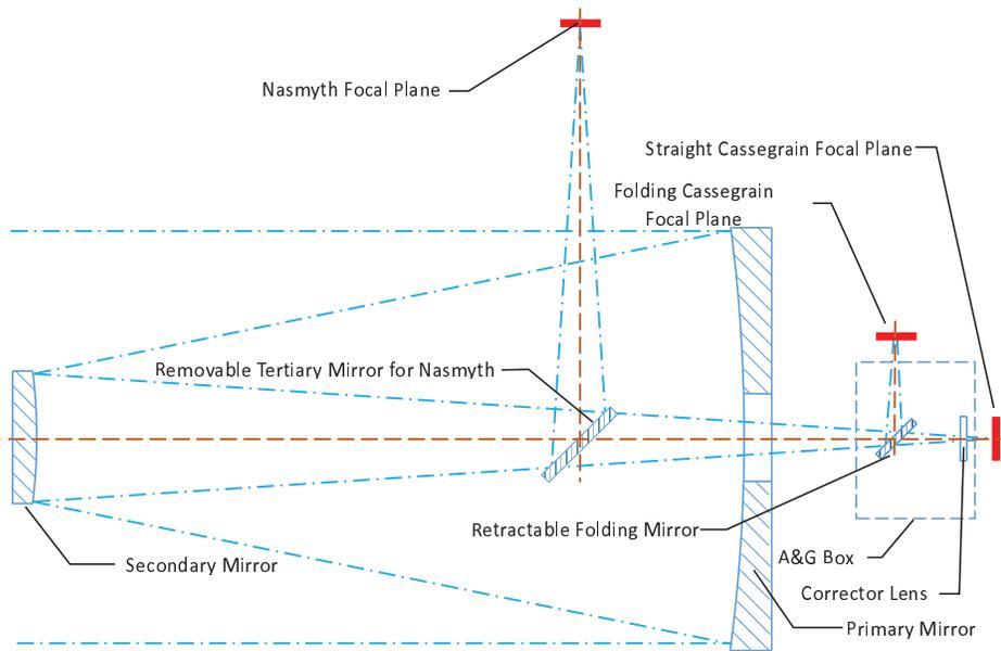
**Fig. 1** The optical layout of the Lijiang 2.4-m telescope, together with the newly added folding mirror for side ports.
