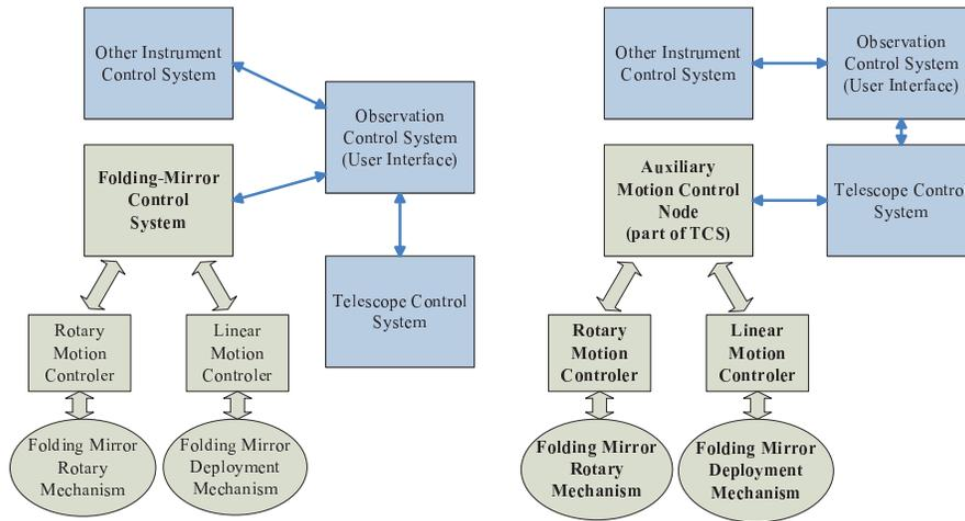
**Fig. 3** Block diagrams of two optional control structures. On the left, the switching system functions in the same way as an instrument, which is controlled directly by the observer. On the right, the folding mirror control is integrated as part of the TCS.
