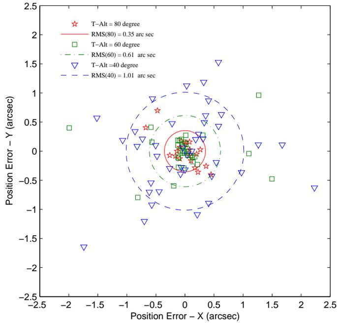
**Fig. 6** The accuracy of RIES tested on PICCD. Each of the red stars, green squares and blue triangles represent the position error measured after one repetition of instrument switching with telescope altitude at  $80^\circ$ ,  $60^\circ$  and  $40^\circ$ , respectively. The red solid, green dash-dotted and blue dashed circles show the RMS of the error with the telescope altitude at  $80^\circ$ ,  $60^\circ$  and  $40^\circ$ , respectively.
