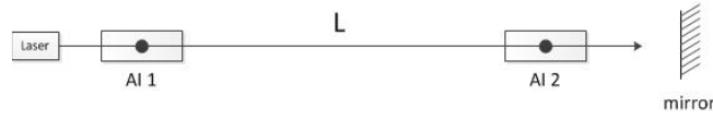
Fig. 6 A schematic of the detector used for gravitational waves that incorporates the new interferometers.
