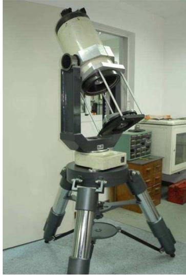
**Fig. 5** Photo of the prototype of a telescope used for atmospheric refraction with double fields of view.
