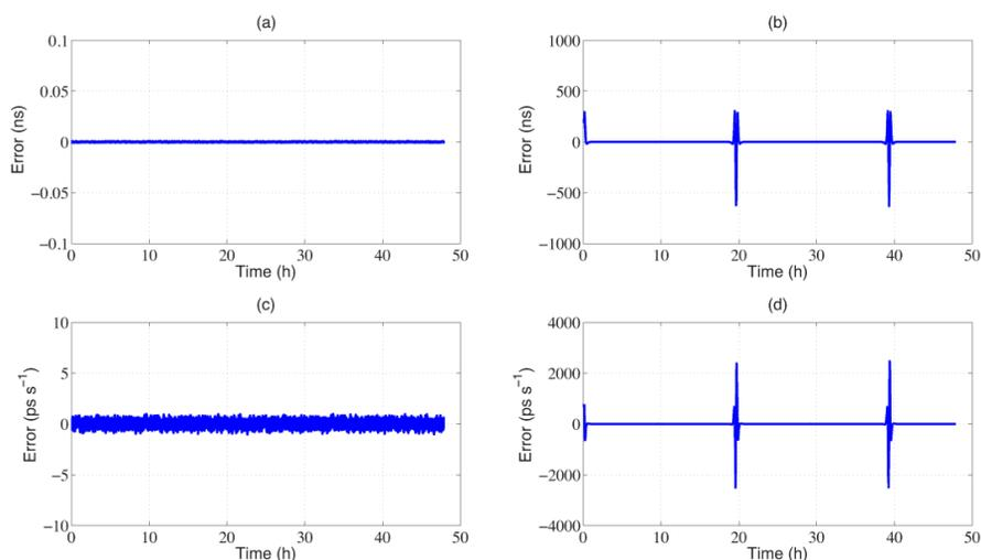
**Fig. 3** The spline fitting error of delay and delay rate of GVLBI (*left*) and C-SVLBI (*right*).
