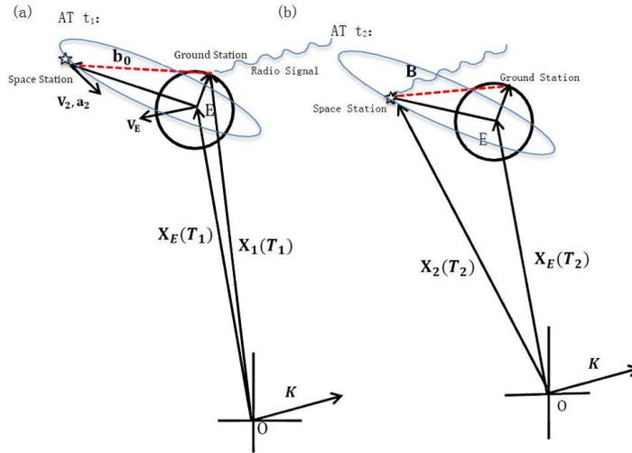
**Fig. 1** Geometry of the receiving stations in SVLBI. (a) The orientation of the signal at the ground station. (b) The orbital movement of the antenna that is part of the satellite at the time the signal is received. The geocenter of the Earth has moved.
