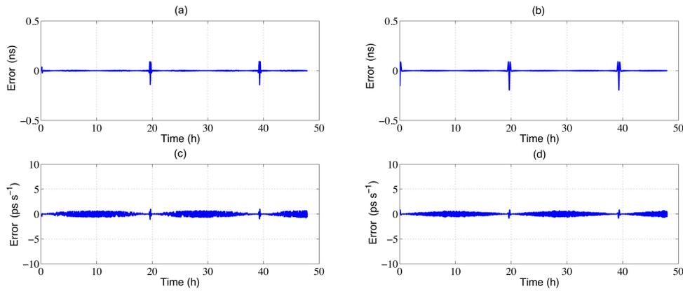
**Fig. 4** The left panel shows the fitting result of a 2 min interval using an 8th-order polynomial. The right panel is the fitting error for a 30 s interval using a 5th-order polynomial.
