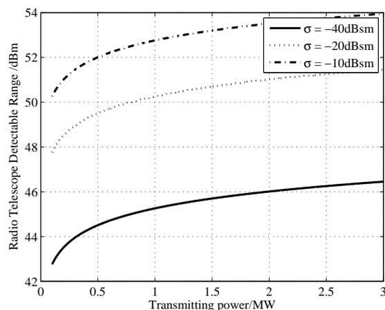
Fig. 8 Detectable range under different transmitting powers.
