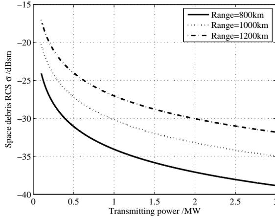
Fig.7 Detectable RCS under different transmitting powers.
