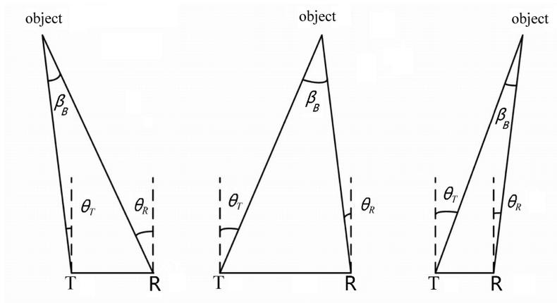
Fig. 1 Spatial relations between positions of the components in a bistatic system.
