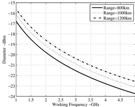
Fig. 6 The relationship between diameter of detectable debris and the working frequency.
