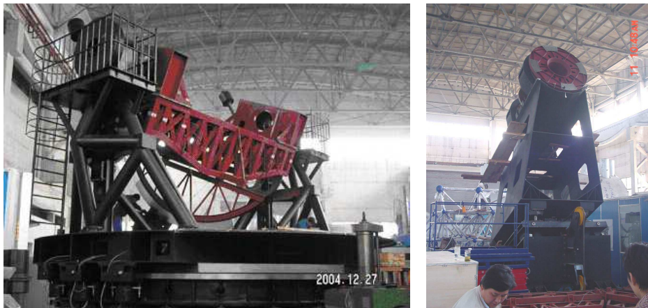
Fig. 23 Left: Ma mounting and tracking structure being assembled; Right: the focal structure being assembled.
