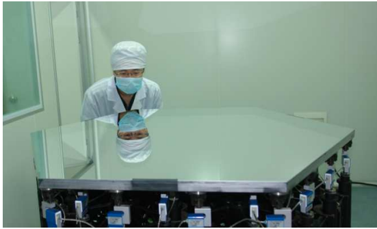
Fig. 18 Ma sub-mirror assembly being tested.
