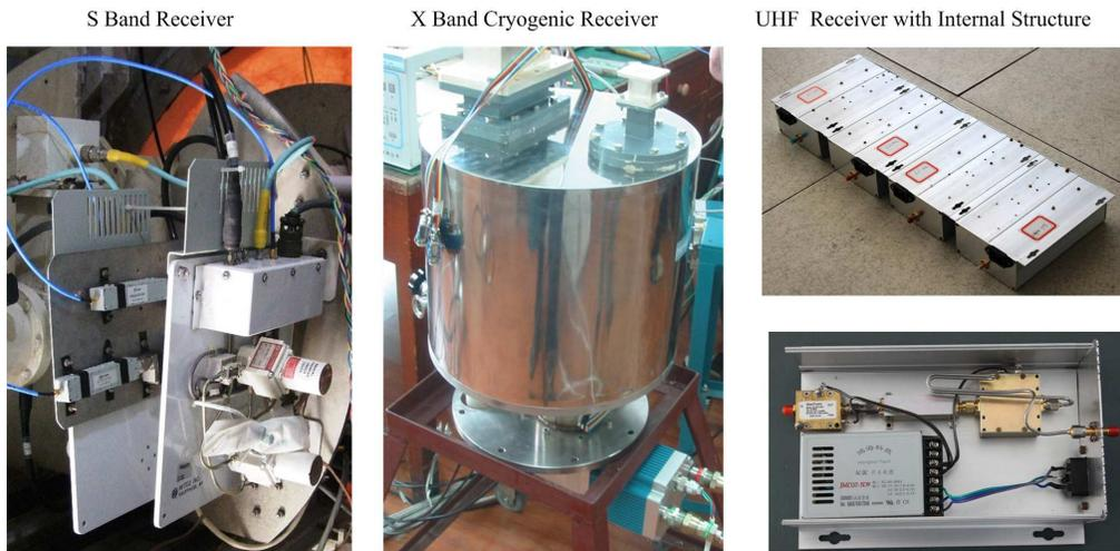
**Fig. 3** Front-end of the IPS observation system.
