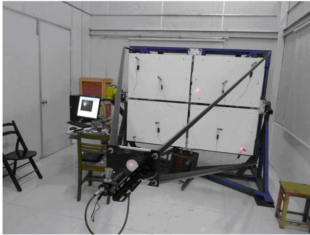
**Fig. 4** Actual equipment of the laser angle metrology system.
