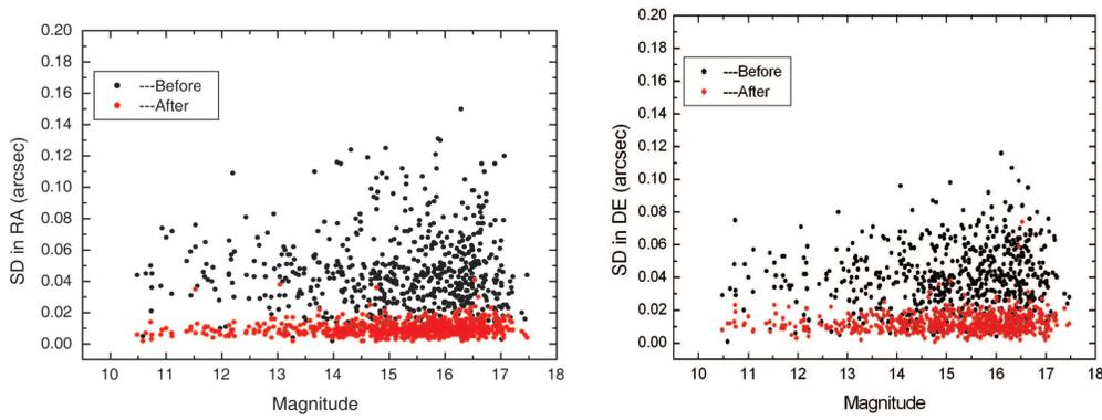
**Fig. 3** Before and after the GD correction, the SD of the star's position ( $O - C$ ) is calculated by the four-constant model. The left is the SD of right ascension and the right is the SD of declination.
