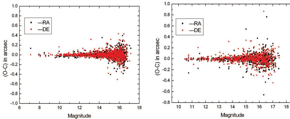
**Fig. 4** ( $O - C$ ) of positional measurement results from two open clusters. The left is from M35 and the right is from NGC 1664.
