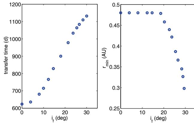
**Fig. 5** Relationship between the minimum transfer time, minimum distance and inclination.
