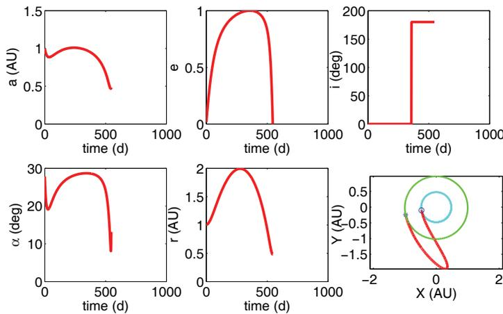
Fig. 4 Optimal reversal transfer trajectory.
