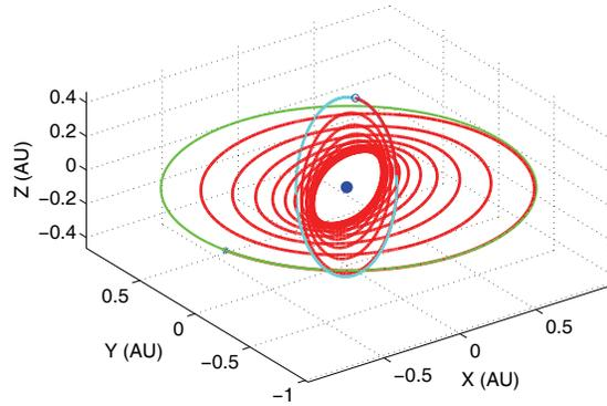
**Fig. 7** Transfer trajectory of  $\beta = 0.058$  for 0.48 AU and a  $75^\circ$  mission.
