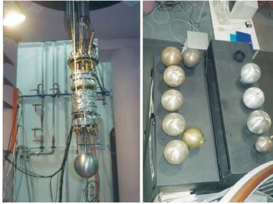
**Fig. 19** *left*: The Dutch setup (dilution refrigerator + sphere + hammer + PZT sensor) for measuring mechanical  $Q$  of small spheres (author's private collection); *right*: Some of the small spheres tested (author's private collection).
