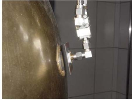
**Fig. 23** Details of the Schenberg pair of microstrip antennae positioned in front of each other. The microwave pump signal from the very low phase noise oscillator jumps from the antenna on the right to the antenna on the left. The later sends the signal to the klystron cavity. Then, the modulated signal jumps back and, thanks to a circulator (which is just above the right angle plug-plug SMA connector), is sent to a cryogenic HEMT preamplifier.
