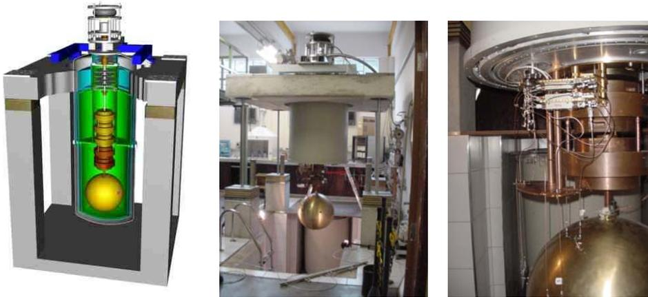
**Fig. 21** Mario Schenberg detector. *left*: Schematic view of the Schenberg detector. Six parametric transducers distributed according to the truncated icosahedron arrangement proposed by Johnson and Merkwitz will monitor their fundamental modes of vibration; *middle*: The Schenberg detector lifted by the hydraulic system; *right*: Details of the antenna with three transducers installed. The three cryogenic HEMT amplifiers are on the top, just below the liquid helium reservoir.
