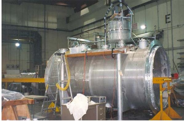
**Fig. 5** Stanford ultra-low temperature detector which was proposed in the late 60s by Fairbank, but never completed (picture taken during the Marcell Grossmann Meeting at Stanford, Palo Alto, in 1994) (author's private collection).
