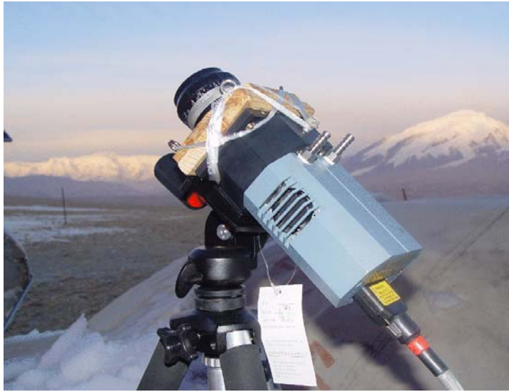
Fig. 4 Andor CCD enclosed in its control box. This picture was taken at Kalasu in the Tajik Autonomous County of Taxkorgan, Xinjiang Pamirs of China.
