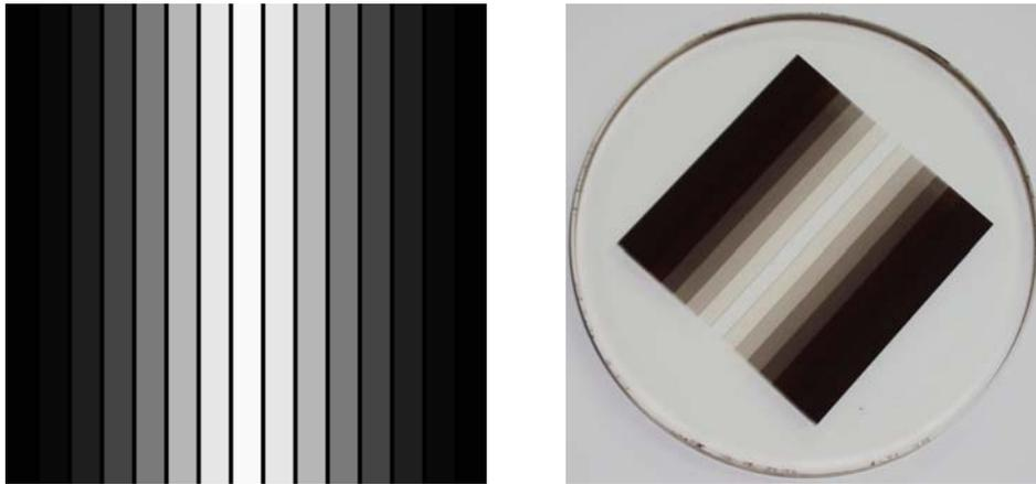
**Fig. 1** *Left*: Transmission amplitude pattern of the newly designed filter, a  $50\ \mu\text{m}$  straight stripe is introduced between each two neighboring steps; *Right*: Photograph of the actual filter.
