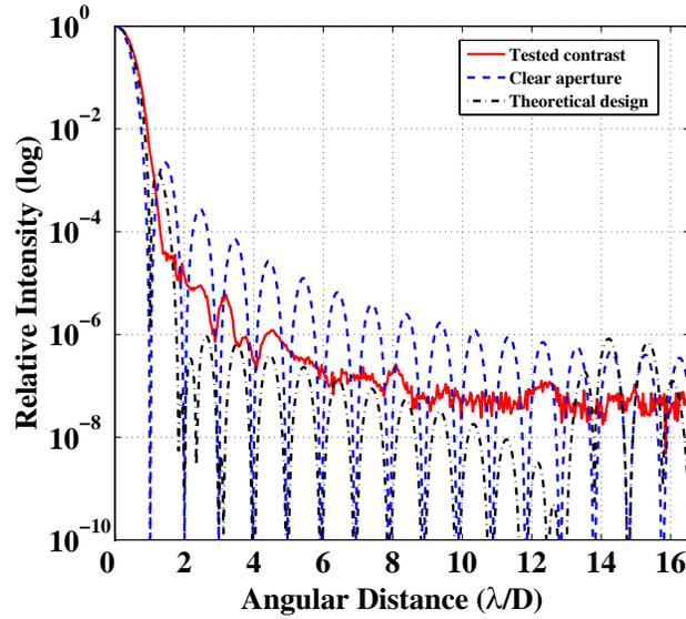
**Fig. 3** Contrast plot along the diagonal direction for a clear aperture (*blue dashed line*), theoretical filter apodization (*black dash-dotted line*) and practical test results (*red solid line*) (see electronic version).
