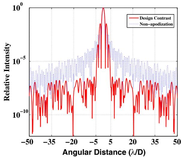
**Fig. 5** PSF contrast plot: a contrast on the order of 10<sup>-6.5</sup> can be achieved in the four diagonal regions.
