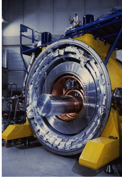
Fig. 2 Generic structure of a resonant solid GW antenna: Example of the antenna “AURIGA” (Legnaro, Italy).
